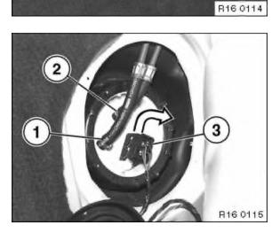
Unfasten hose clip (1/2) with special tool and remove hoses. Unlock connector (3) and remove.
